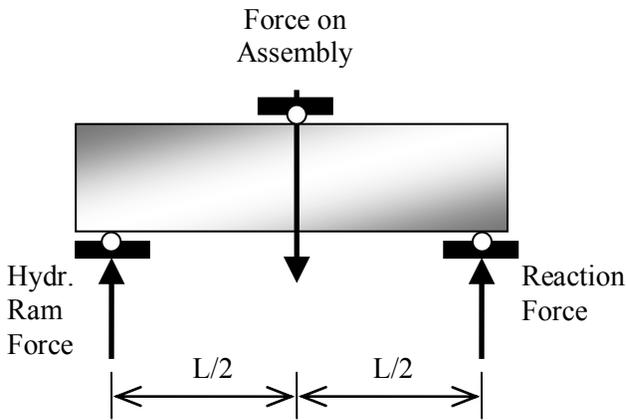
a) Force Leverage Concept at Top Beams
