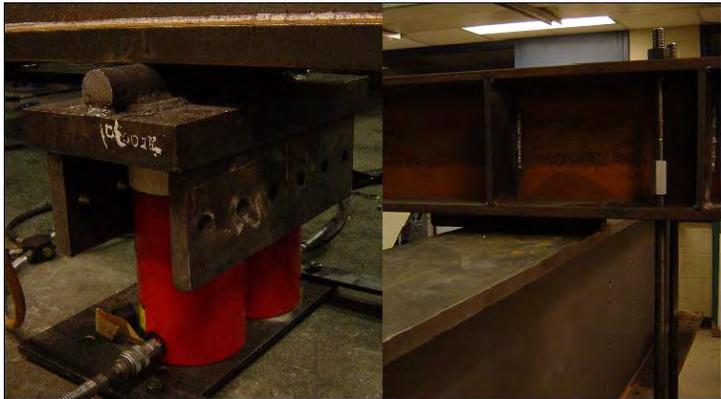
**Figure 18:** Applied loading points for girder splice test.
