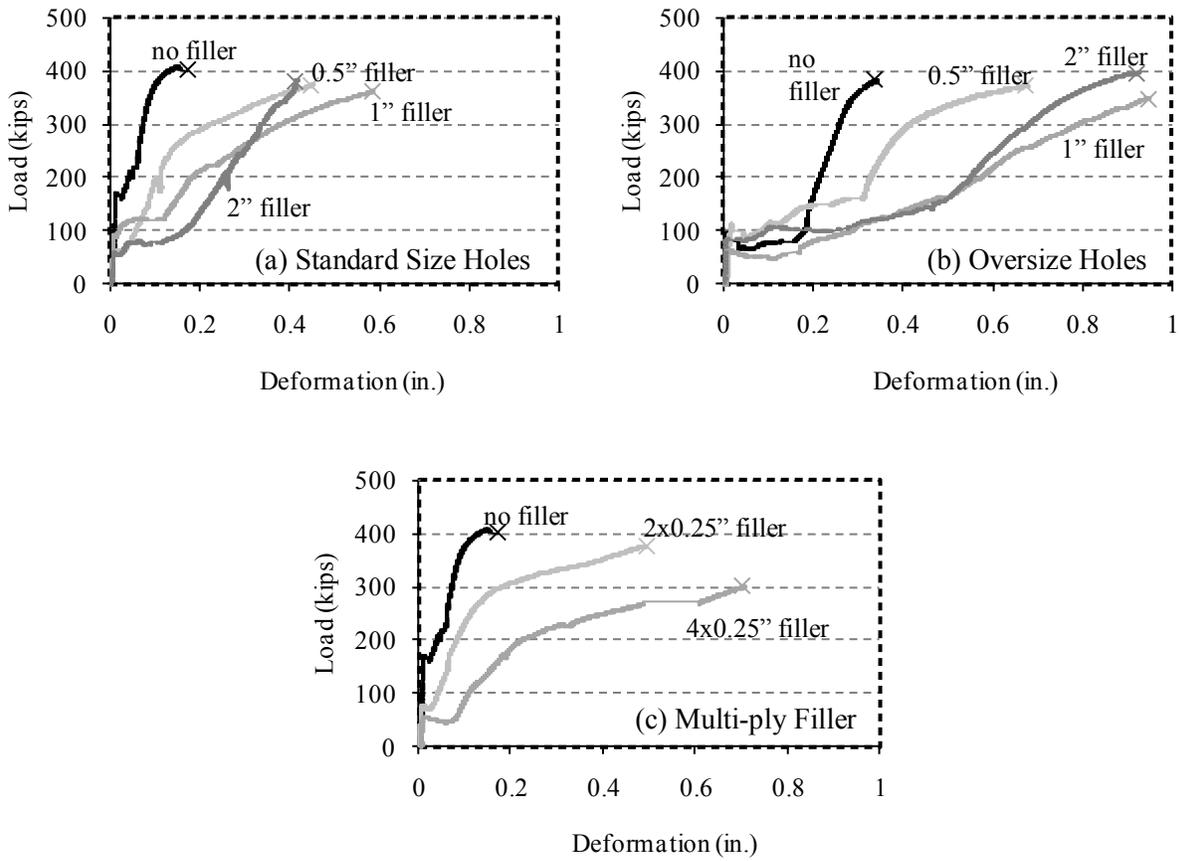
**Figure 7: Examples of Three-bolt Assembly Force Deformation Results**
