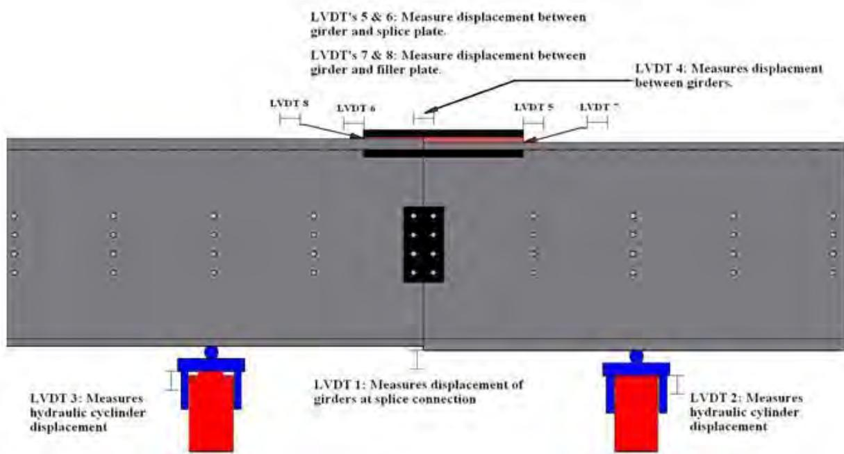
**Figure 20:** LVDT layout on the test apparatus
